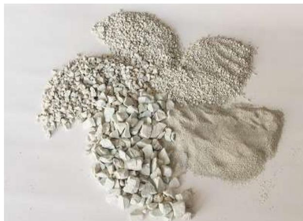
Figure 3. Zeolite mineral used as a sorbent
